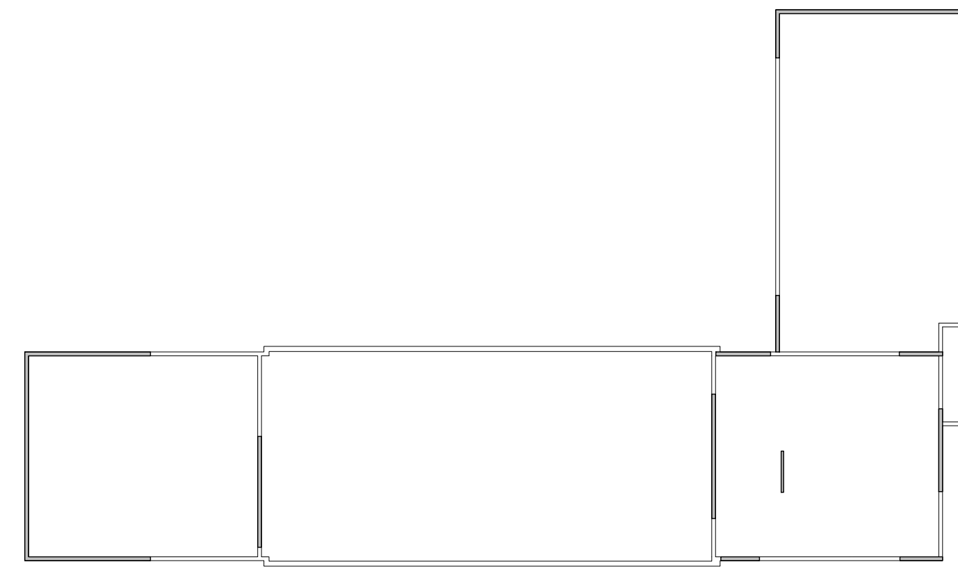
SHEARWALL LAYOUT PLAN ABOVE FIRST FLOOR COORDINATE WITH LOCATION OF HOLD DOWNS
